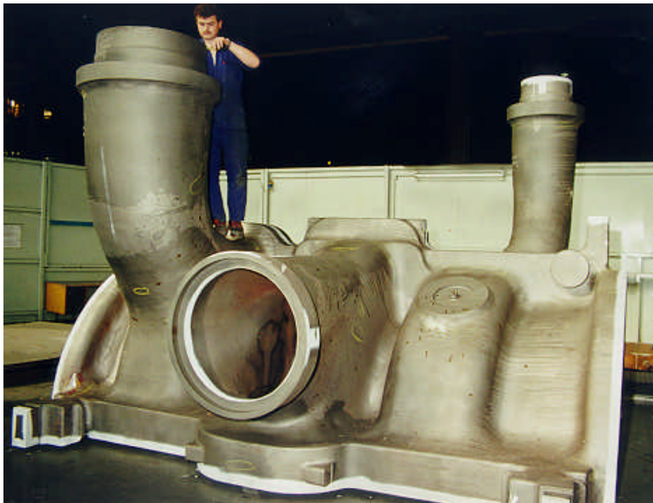
Figure 13: Project Schwarze Pumpe, IP Innenr Casing, 40 t with welded on, cast elbows (G-X 12 CrMoWVNbN 10 1 1)
