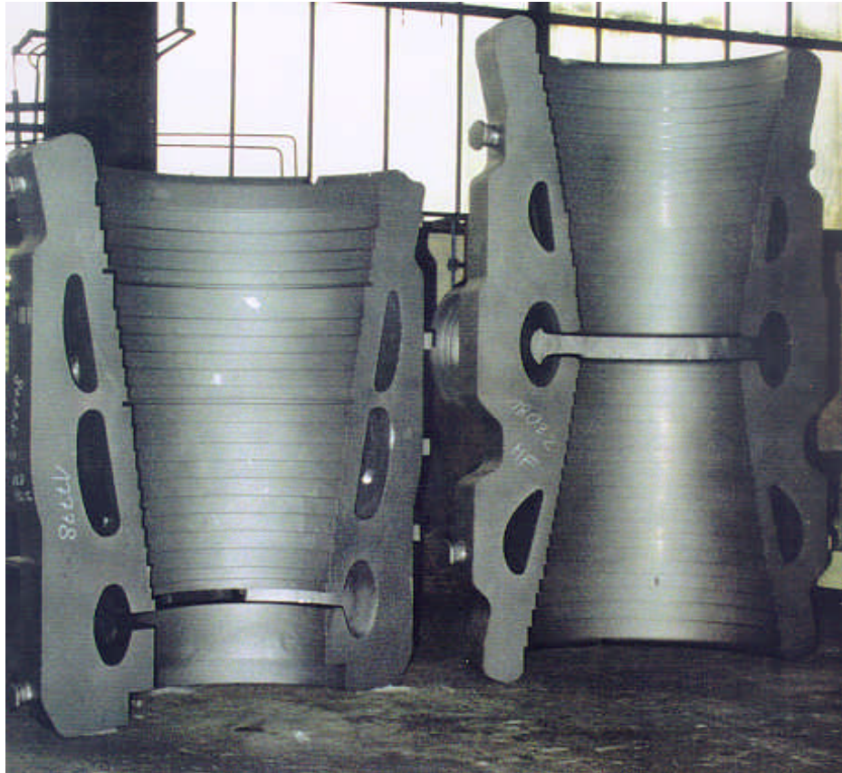
Figure 12: Projects Schkopau and Meri Pori IP Innenr Casing, 14 t and 19 t (G-X 12 CrMoWVNbN 10 1 1)
